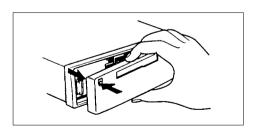
If the set was still in operation, it will turn off now. All current settings remain stored. If a cassette is inserted, it will be kept in the set. The radio will turn on automatically when you attach the release panel again.
